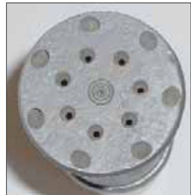
Illustration of base of leaflet rocket. Note the percussion cap in the centre of the rocket and the slanted venturi at the rim.
